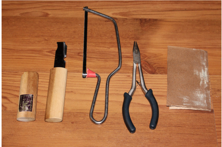
Figure 89: Basic shinai repair toolkit.
