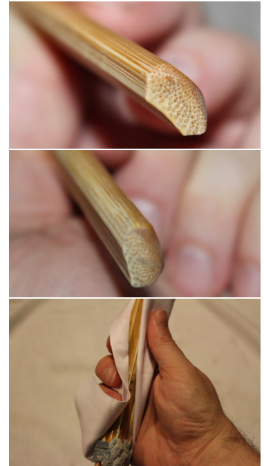
Figure 81: (Top) Un-sanded slats have pointed edges, (Center) after light sanding the edges are rounded. (Bottom) Use a cloth to rub oil onto the slats.
